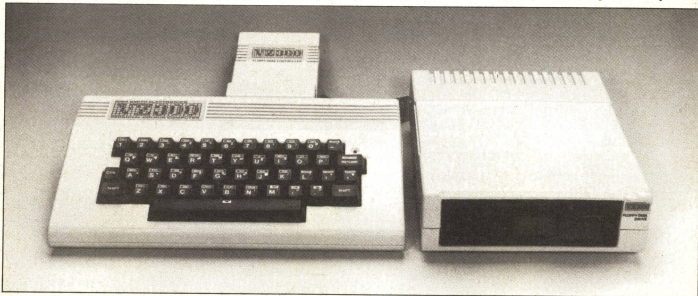
The VZ300 Computer with the DOS (disk operating system) cartridge plugged in at the rear. It, in turn, has a "piggyback" socket for RAM or ROM modules. On the right is the VZ300 Floppy Disk Drive.
